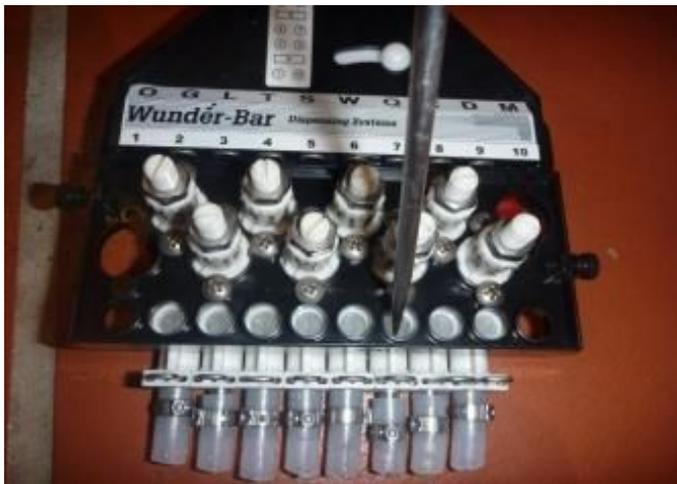
2. For this example we are referring to Q Flow Control (Squash). Use a Philips head screwdriver, and then slowly undo the closet screw to you. Some product will drip, but not under pressure if you have followed step 1 correctly.
