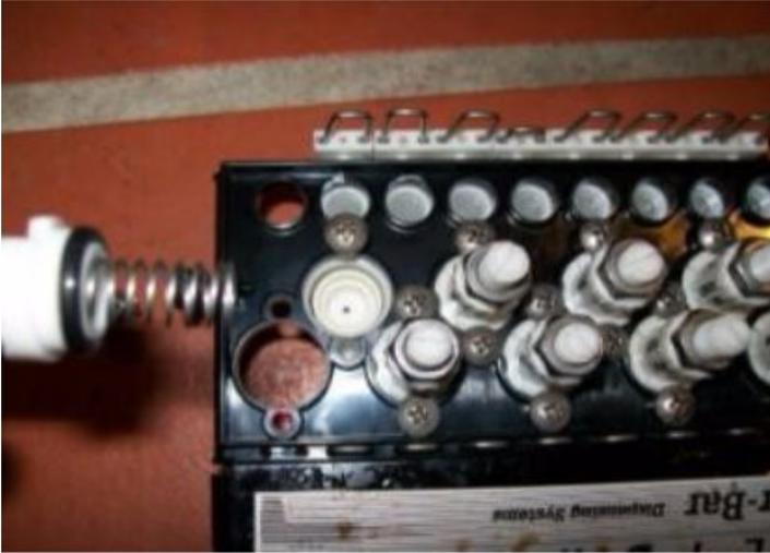
5. Remove the 2 ceramic sleeves. Note the O Ring in the base of the manifold. Leave this.
