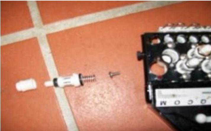
7. Before washing these items. Make note of how the inner sleeves hole faces downwards and the outer sleeve holes face upwards and how one sits inside the other.
