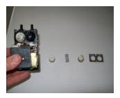
Now the 2 ceramic sleeves maybe stuck together. Simply wash in cold water so that eventually you can slide the inner sleeve inside the outer sleeve.
